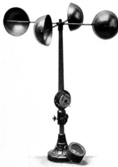
THE ROBINSON ANEMOMETER.
