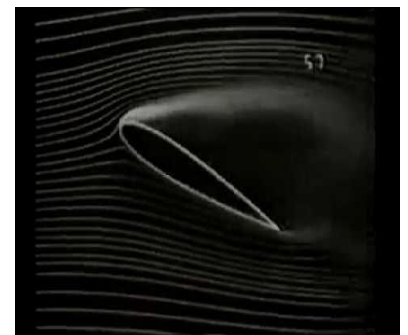
Separated Flow at Critical \alpha
