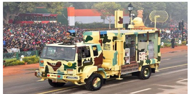
Mobile Base Transceiver Station
