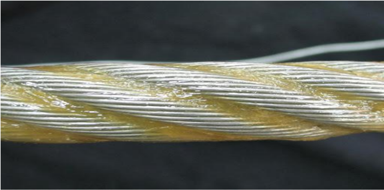
Greasing of Steel Wire Rope
